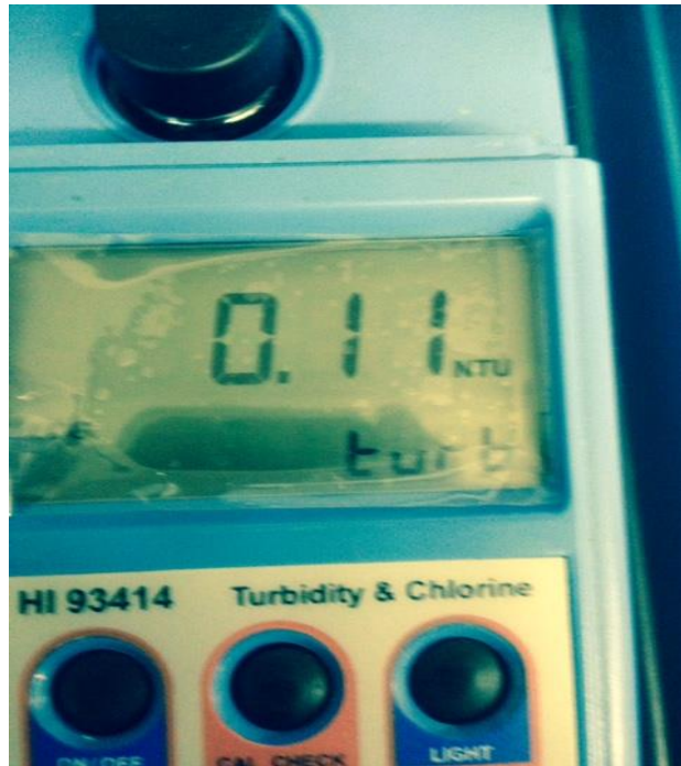
Figure 4.23 : Monitoring the Turbidity of the treated effluent
