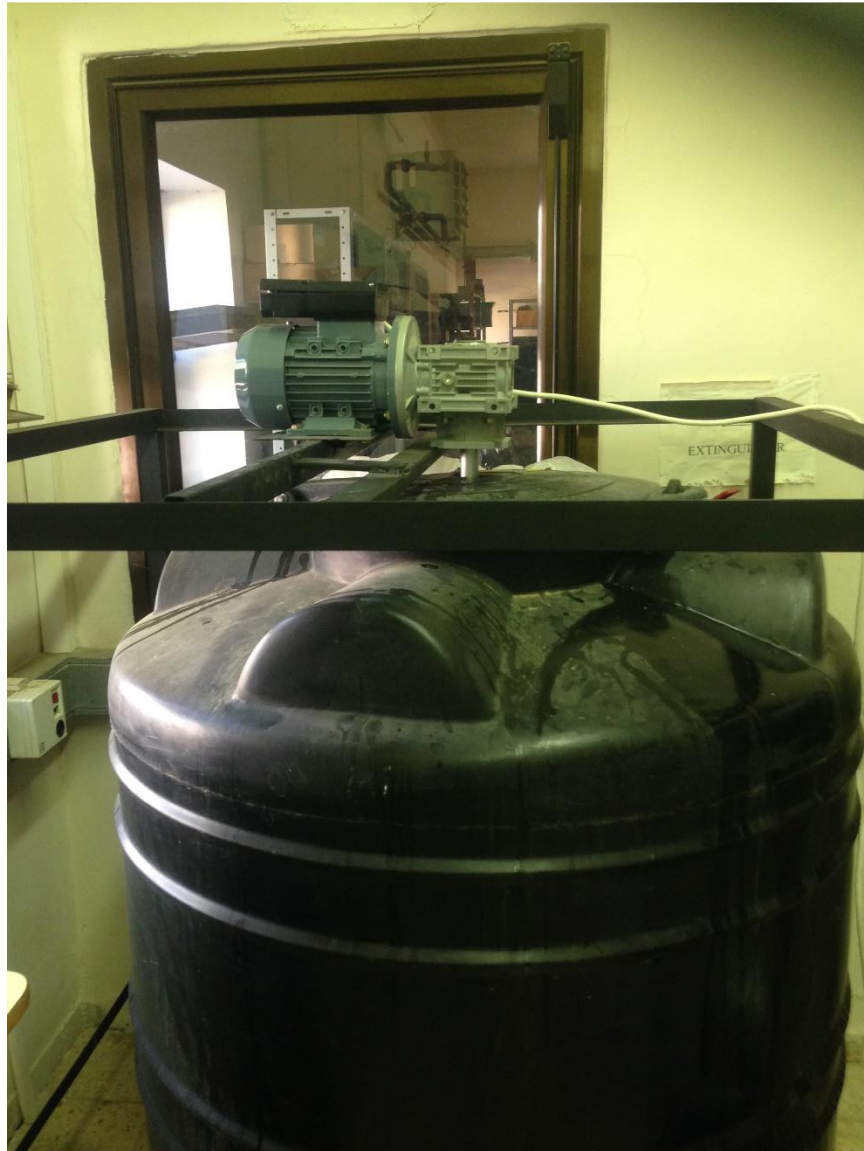
Figure 3.3: The 1000 L feeding tank with mixer
