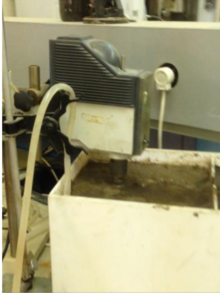
Figure 3.5: Variable speed mixer
