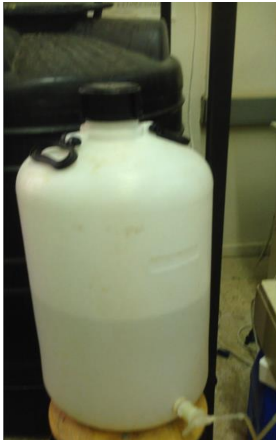
Figure 3.2: Feeding tank with capacity 50L
