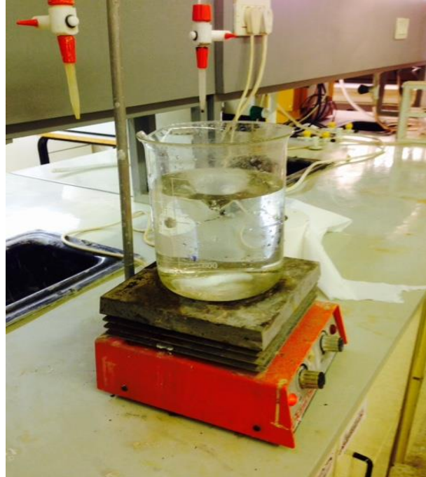
Figure 3.6: Mixing the \text{KNO}_3 with tap water
