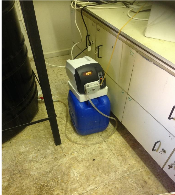
Figure 3.8: The Peristaltic pump that was used during the test
